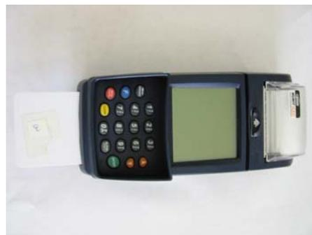
**Overhead view of Lipman Nurit Device with test Smart Card**
